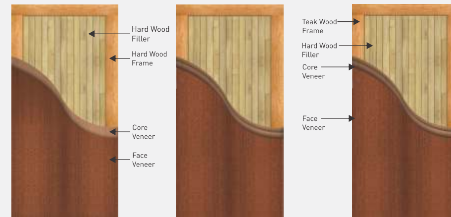
Hard Wood Frame- Single Core 5 Ply Construction
